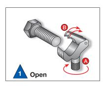
Turn handle (A) to raise floating blades (B). Place the Nes External tool over thread to be repaired.
