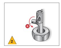
Turn knurled knob **K** to extend blade **B** into a thread groove on an undamaged section and tighten by hand only.
