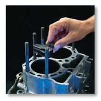
▲ The **Nes External** thread restorer is available in 3 sizes and can repair threads from 4 mm (5/32") diameter up to 128 mm (5") dia.
