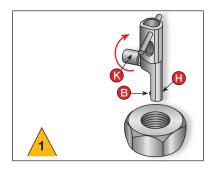
Turn knurled knob **K** to fully retract the blade B into the housing **H**. Insert **Nes Internal** tool into the threaded hole or bore to be repaired.
