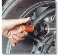
The Nes Internal thread restorer is available in 6 sizes and can repair threads from 8 mm (5/16") diameter up to 68 mm ( 2 5/8") diameter.
